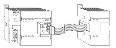
The ribbon connector is protected by a cover on the base unit. Side-by-side mounting completely encloses and protects the ribbon connector.
