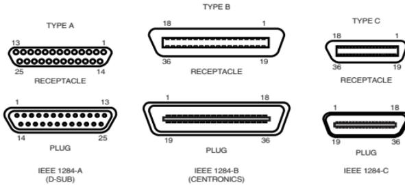
The three different types of IEEE-1284 parallel port connections. Type A receptacle (DB-25m) is used on computers; Type B receptacle is used on most printers. Some HP LaserJet printers use both Type B and Type C receptacles.
