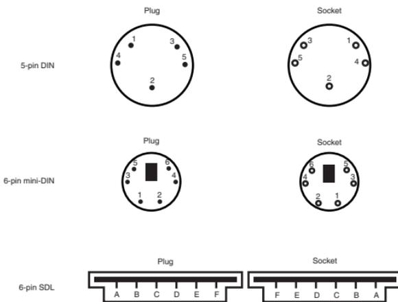
**Figure 9.4** Keyboard and mouse connectors.
