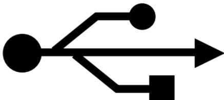
**Figure 8.1** This icon is used to identify USB cables, connectors, and peripherals.
