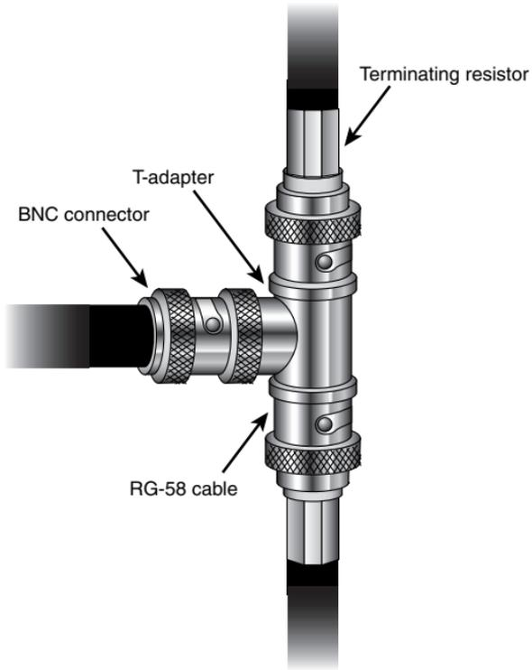
The BNC connector with T-adapter, resistor, and BNC (RG-58 Thin Ethernet) cable.
