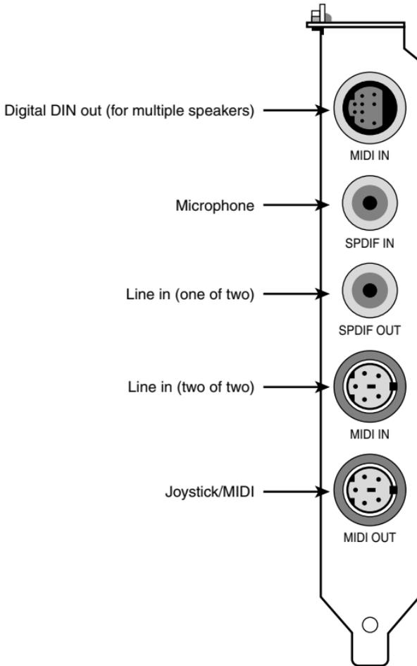
Some or all of these ports—digital DIN, SPDIF in, SPDIF out, MIDI in, and MIDI out (top to bottom)—can be found in various combinations on advanced sound cards. They can be mounted on a daughtercard bracket (shown here), attached to the rear of the sound card itself, or mounted on a box connected to the outside of the computer.
