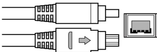
Some IEEE-1394 devices use a four-wire cable and receptacle instead, omitting the power lines.
