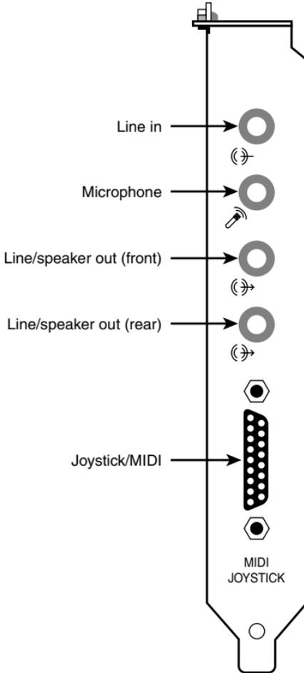
Speaker out, microphone, dual line-in, and MIDI/Joystick port (top to bottom) are found on typical sound cards of all types.
