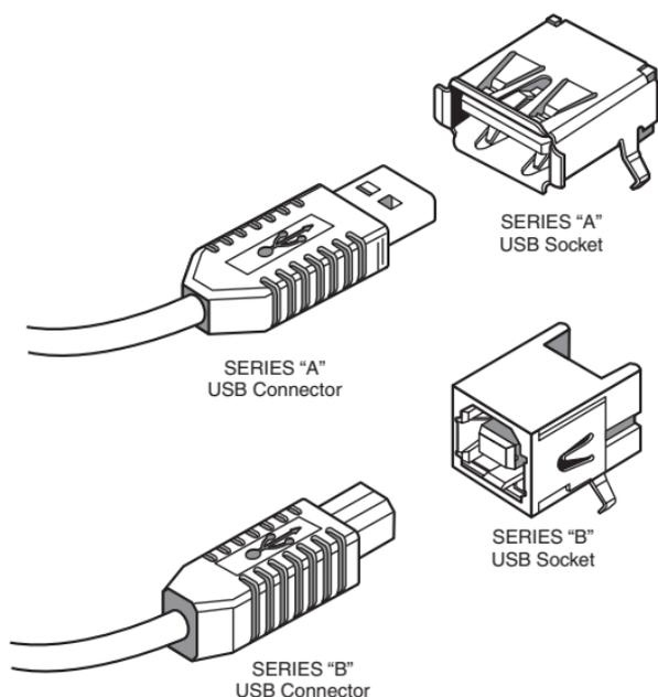
**Figure 8.2** USB Series A and Series B plugs and receptacles.
