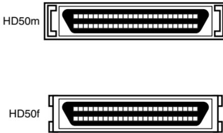
The SCSI HD-50m cable connector (top) and HD-50f receptacle (bottom) are the most common types of external SCSI ports used today.
