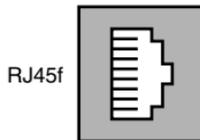
An RJ-45 port, typically used for UTP Ethernet/Fast Ethernet.
