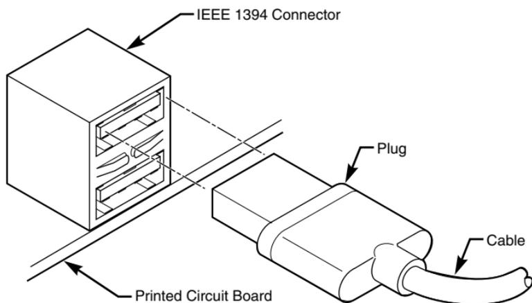
The standard 6-wire IEEE-1394 (FireWire, i.Link) connector, receptacle, and cable.
