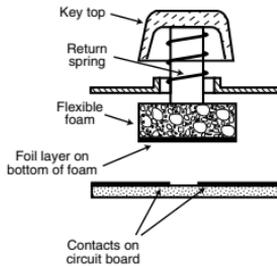
**Figure 9.1** A typical foam-element mechanical keyswitch.
