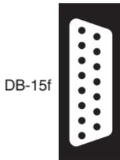
A DB-15 connector used for Thick Ethernet (10BASE-5) networks; usually found on the rear of a network card along with an RJ-45 or a BNC connector.
