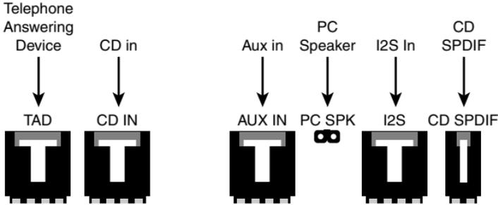
Typical internal sound card ports include, from left to right, TAD (telephone answering device for use with modems), CD in (for playing music CDs through the sound card speakers), Aux in (for connecting other devices), PC SPK (for playing PC speaker beeps through the sound card's speakers), I2S in (for playing DVD audio), and CD SPDIF (for playing digital audio from CD-ROM drives with SPDIF output).
