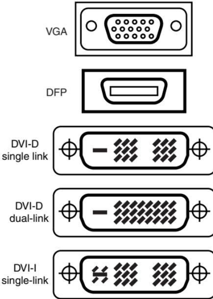
VGA, DFP, DVI-D single link, DVI-D dual link, and DVI-I video cable connectors (top to bottom).
