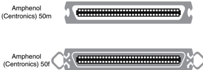
The traditional (Amphenol/Centronics) 50m cable connector (top) and 50f receptacle (bottom) are still widely used for external SCSI devices.
