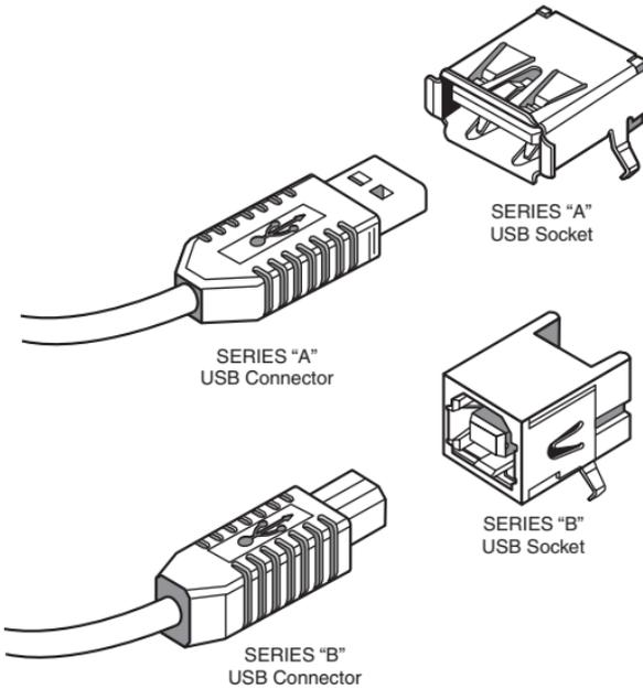
USB Type A and Type B ports and cables. Use a Type A to Type B cable to run between USB hubs and most USB devices.
