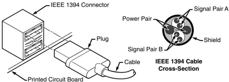
**Figure 8.3** IEEE-1394 cable, socket, and connector plug.
