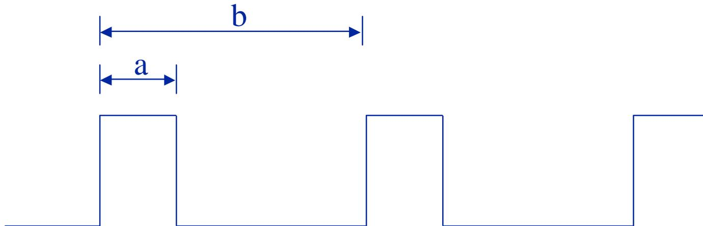
$$\text{Duty cycle} = \frac{a}{b} \times 100\% \quad \text{Freq} = \frac{1}{b} \quad (\text{usually constant})$$
