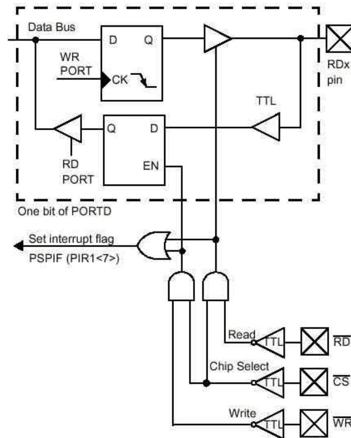
Note: I/O pin has protection diodes to VDD and Vss.
